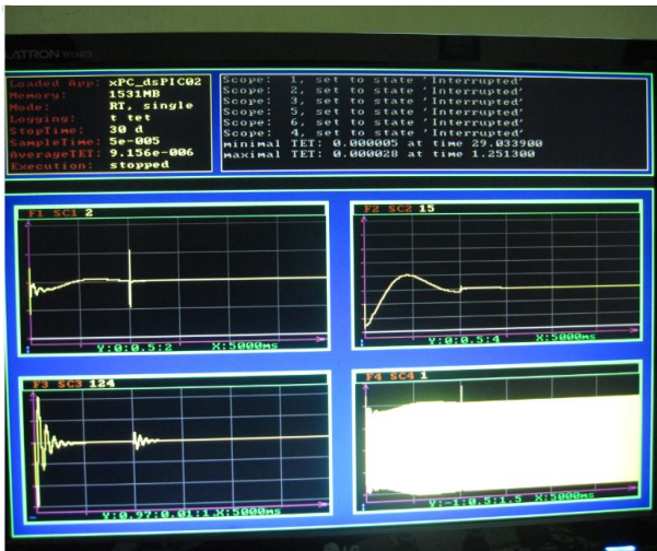
Fig. 12. The excitation response in target PC
