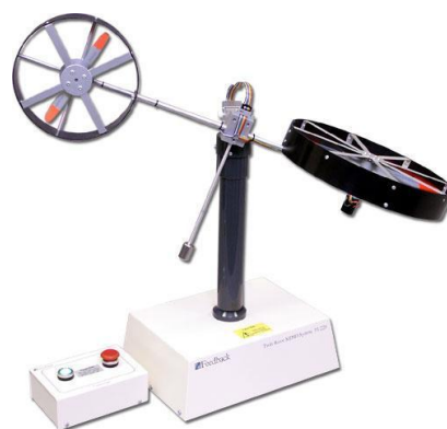
H.1. Twin Rotor MIMO System
